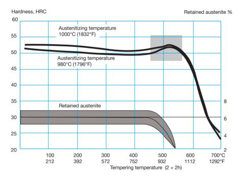
Above tempering curves are obtained after heat treatment of samples with a size of 15 x 15 x 40 mm, cooling in forced air. Lower hardness can be expected after heat treatment of tools and dies due to factors like actual tool size and heat treatment parameters.
