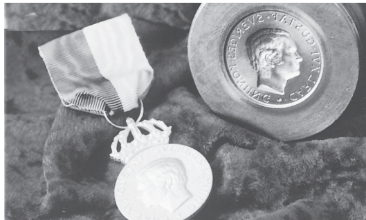
Cold work product where Uddeholm Calmax would be a good choice for the die.
