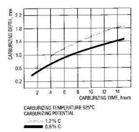
The carburizing depth is the depth that corresponds to a carbon content of 0.3%.
